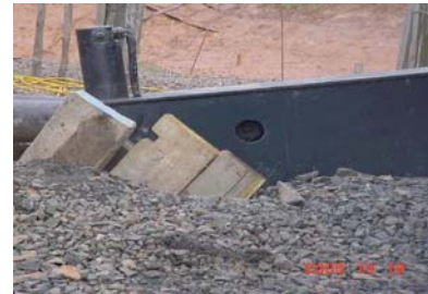
Outrigger punched through the ground
